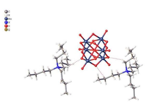
Single crystal XRD showing 6 MoO6 octahedra. Each polyanion hydrogen bonded to two counter cations Exhibits Lindqvist arrangement.
